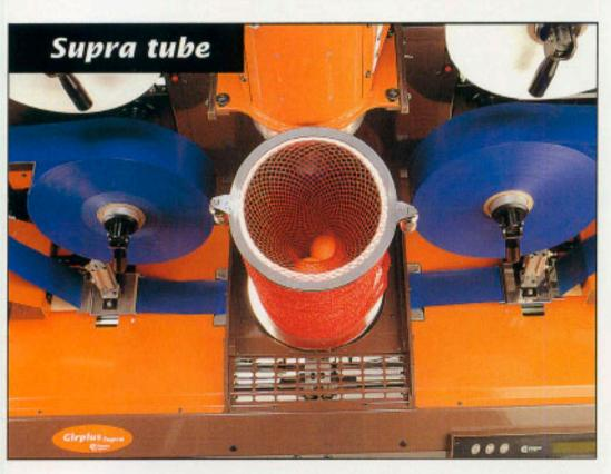
The new design net tube feeds the net from the top of the tube, so that the fruit is received directly into the net and is controlled as it is rapidly transported to the welding position ensuring the possibility of damage is eliminated.
